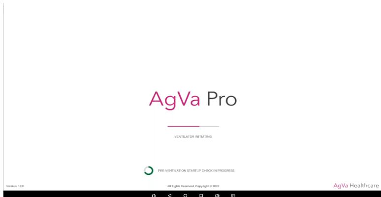
Upon starting, the AGVA PRO logo and a labelled progress bar will appear. Once loading is finished, the message “sensors check success, ventilation can be started” will appear.
